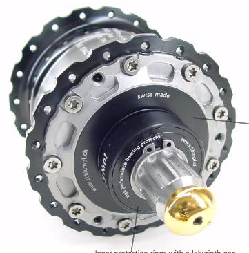
Outer protection rings with a labyrinth gap of 0.1mm guard against entry of dust or spray water.
