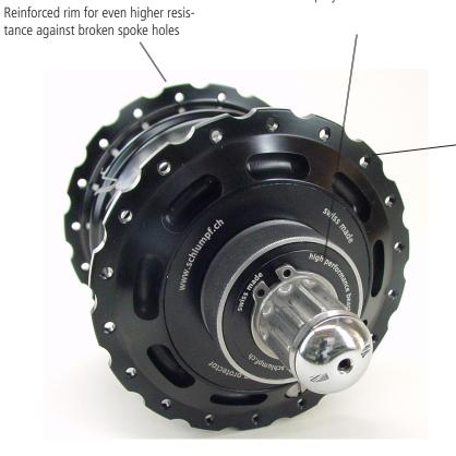
Countersunk parts on both sides of spoke holes: spokes can be fitted from both sides. No danger of wrong installation.
