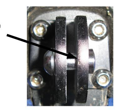
**Solution**: the hole for the hex bolt needs to be re-drilled to 8 mm diameter (or 5/16").
